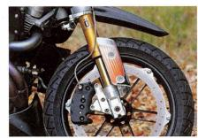
The fully adjustable Öhlins fork was originally intended for Buell's controversial XBRR Formula Xtreme racebike. A custom lower right leg accommodates the massive eight-piston Nissin brake caliper
