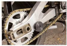
The chain-drive conversion swingarm from the old Buell race kit is now available through Erik Buell Racing, replacing the OEM belt drive and allowing easy gearing changes. It looks trick, too.
