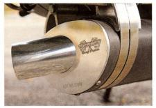
Polished stainless-steel end cap is the only indication the muffler has been modified by Drummer. It's 7 lbs. lighter, makes 8 lb.-ft. more torque and triggers car alarms at nine paces
